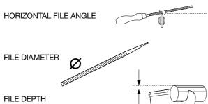
See "Technical Specifications" for the details which apply to your chain. It is very difficult to file a chain saw correctly without the proper aids. We recommend the use of a file guide to ensure maximum cutting efficiency with the least tendency to kickback.
